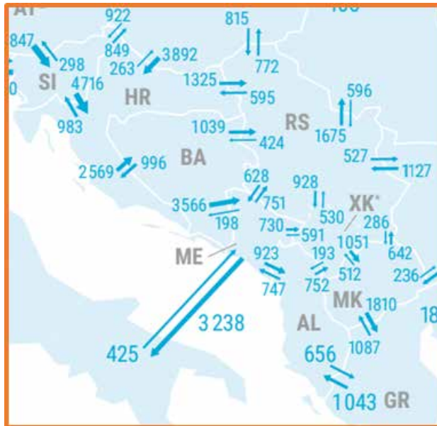
Figure 6. Cross-border transmission capacity and regional energy flows.
